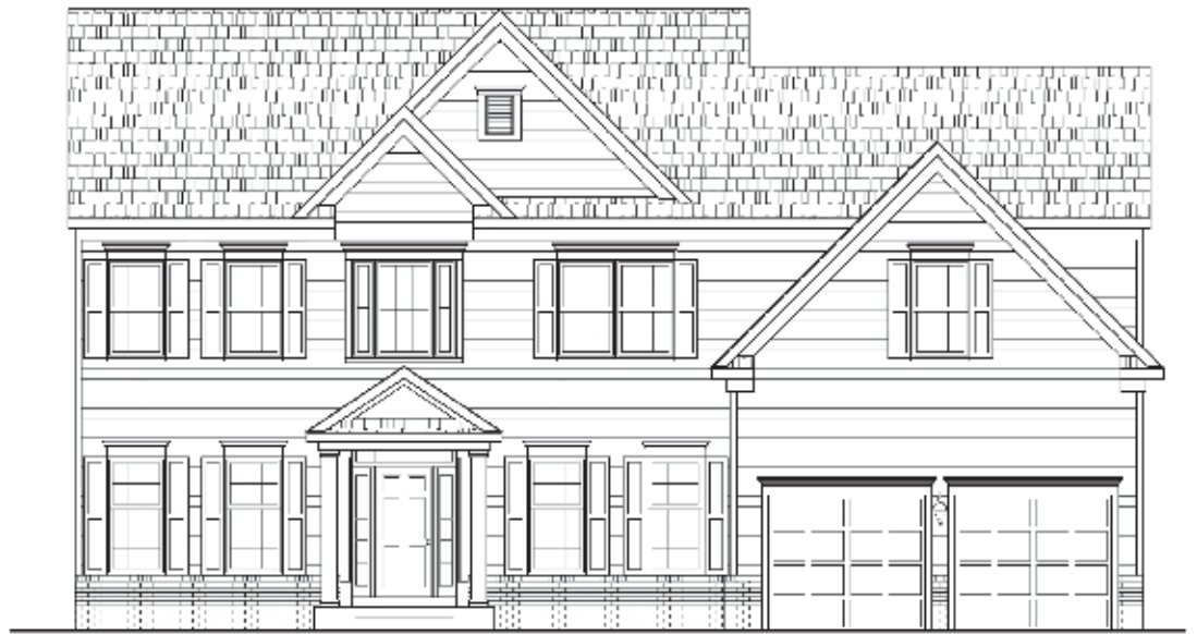
Elevation 1 with Brick Water Table
